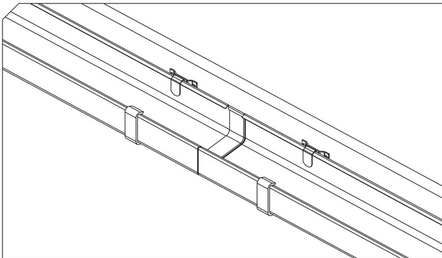
**Figure 6. Adjacent brackets not farther than 15 cm from glued joints**
