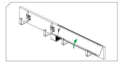
4. Attach one gutter to the brackets and the connector.
