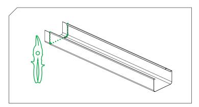
3. Use sheet metal scissors to cut off the stamped tip of the gutter that is to be placed in the connector.
