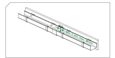
6. Leave a 5-10 mm expansion gap between the gutters.
