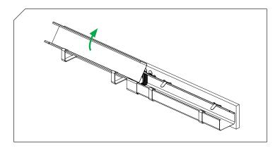
5. Attach the other gutter to the brackets and the connector.
