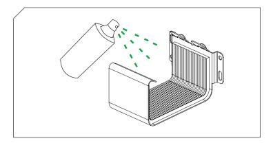
Prior to inserting the gutter into the connector, spray the gasket with a lubricant spray!
