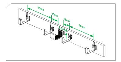
In order to ensure proper adhesion of the gutter bottom to the gasket, the connector should be raised by approx. 1-2 mm in relation to the level of adjacent brackets.
