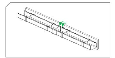
7. Fold the mounting plates of the connector.
