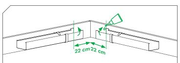
Lift the notched drips of the gutters to vertical position. Cover the area where the corner is to be placed with two lines of adhesive (1.5 cm from the gutter edge).
