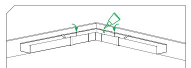
Fold the drips of the gutters on the corner. Secure the connection from the inside using sealing glue.
