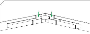
Insert the corner in the gutters previously covered with sealing glue.
